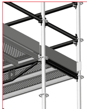
Rys. 3.24 – Corner formed of two stands
