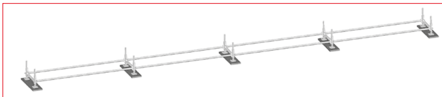
Rys. 3.54 – Step 3 - Tying the initial components
