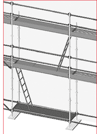
Rys. 3.41 – Scaffolding entrance with passing aluminium platforms fitted with the aluminium ladders
