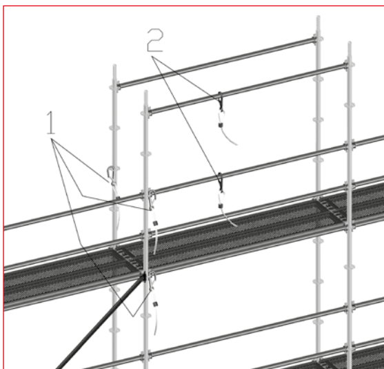
Rys. 3.8 – Personnel Protection Equipment attachment points
