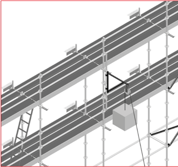
Rys. 3.79 – Scaffolding with the winch
