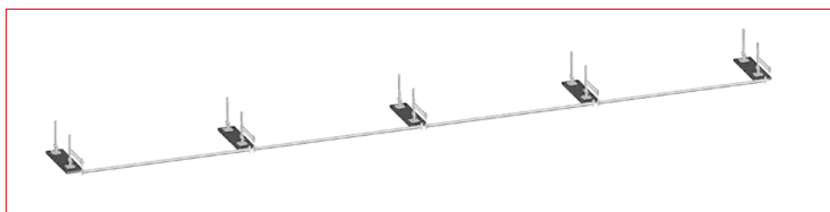
Rys. 3.52 – Step 1 – Footing assembly
