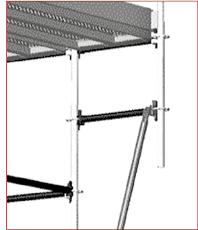
Rys. 3.29 – Platform expanded with the transoms and braces
